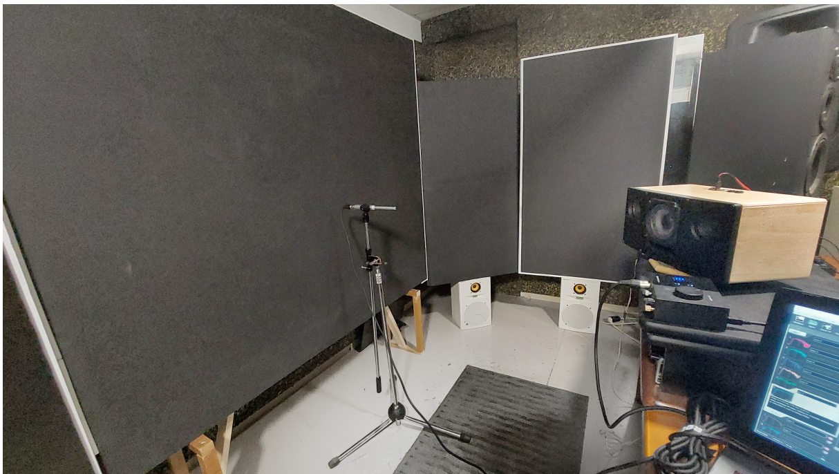
Figure 5.41: Measurement process with the microphone placed 1m away from the speaker
