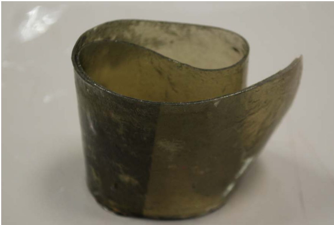
Fig. 1. One of the letters of the word Silere showing the strong yellowing and opacity of the polymer.
