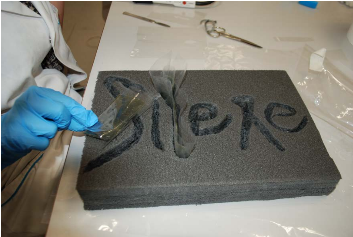
Fig. 4. You can see how the lettering is coated with Melinex® and the contrast between its transparency and the yellowish tone of the lettering.
