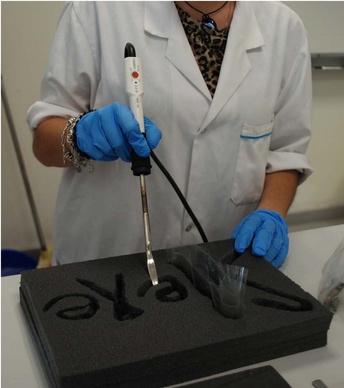
Fig. 2. When adjusting the exact shape of the letters thanks to the hot spatula.
