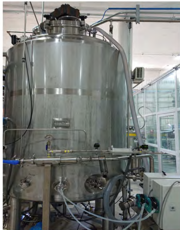
Figure 8. Mixing tank for preparation of formulations in the Punta Delicia plant.
