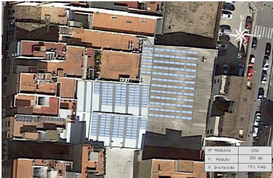
Figure 66. Proposal B, all modules facing south. In addition, modules on the north water with structure to rectify them to south orientation as well. Source: Own creation.
