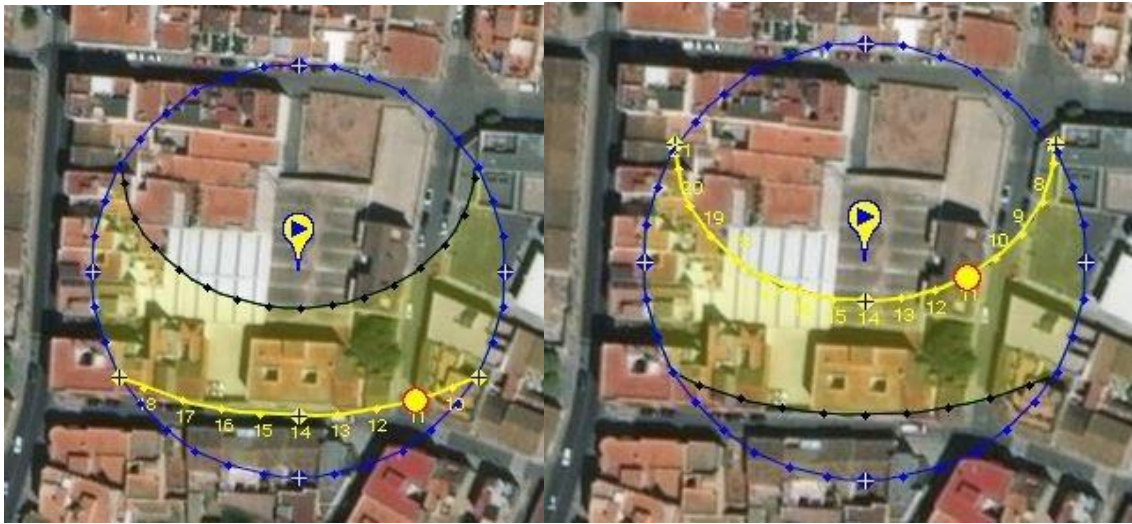
Figure 50. Fan of the solar position according to times of day and days of the year. Left: 11:00 am on the day of the summer solstice (21 June); Right: 11:00 am on the day of the winter solstice (21 December). Source: Sun Earth Tools (Web application).
