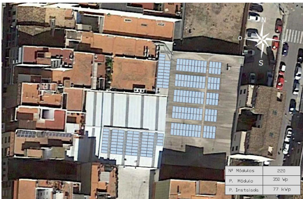
Figure 67. Proposal C, south facing modules on the white roof and east-west facing modules on the brown roof. Source: Own creation.
