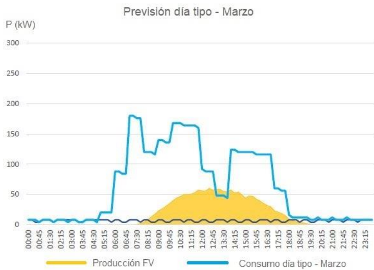
Figure 125. Graph of PV production and consumption forecast, for a standard working day in March. Source: Own creation.
