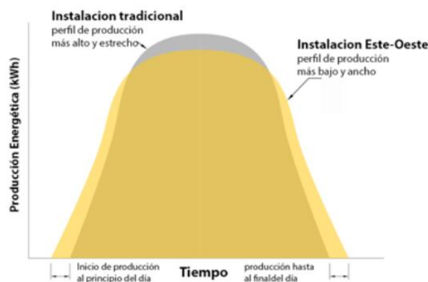
Figure 74. Effect of the widening of the PV production curve in an east-west installation. Source: MonSolar
