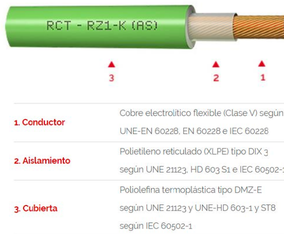
Figure 107. RZ1-K (AS) 0.6/1kV single-pole cable for AC side. Source of supply: RCT cables.
