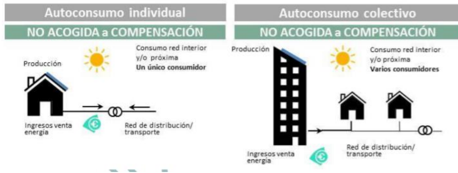
Figure 37. Diagrams of self-consumption WITH surplus NOT eligible for compensation, left: individual; right: collective. Source: IDAE: Guía del Autoconsumo, 2019.
