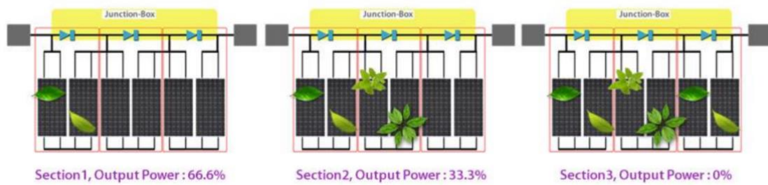
Figure 28. Schematic diagram of bypass diode operation. Source: Own
