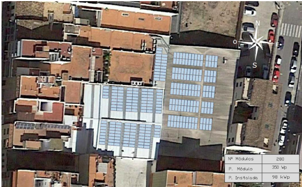
Figure 68. Proposal D, south facing modules on the white roof and east-west facing modules on the brown roof. In addition, modules on the north water with structure to rectify them to south orientation. Source: Own creation.
