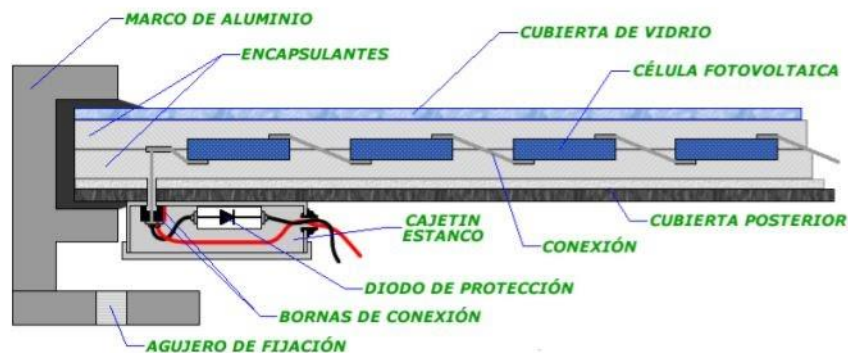
Figure 26. Parts of a conventional PV panel. Source: Own creation
