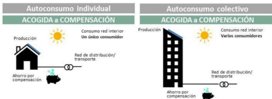
Figure 36. Diagrams of self-consumption with surpluses receiving compensation, left: individual; right: collective. Source: IDAE: Guía del Autoconsumo, 2019.
