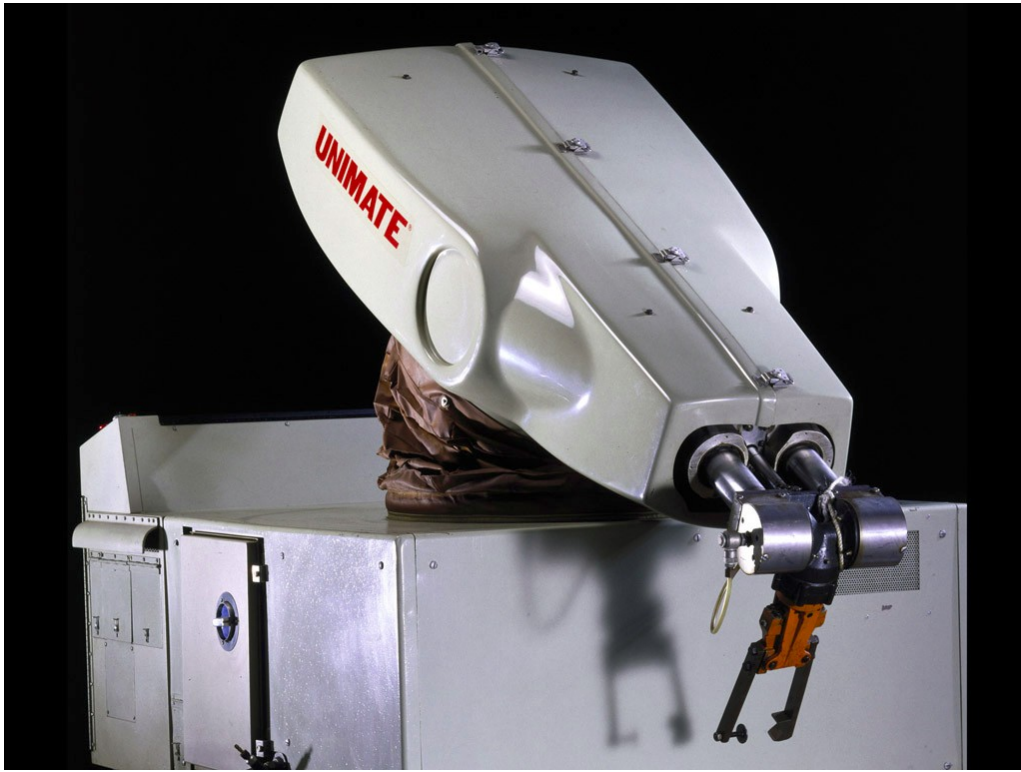
Figure 4 The Unimate was the first industrial robot ever built. It was a hydraulic manipulator arm that could perform repetitive tasks. It was used by car makers to automate metalworking and welding processes.
