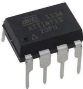
Figura 43. Atmel ATtiny13-20PU.
