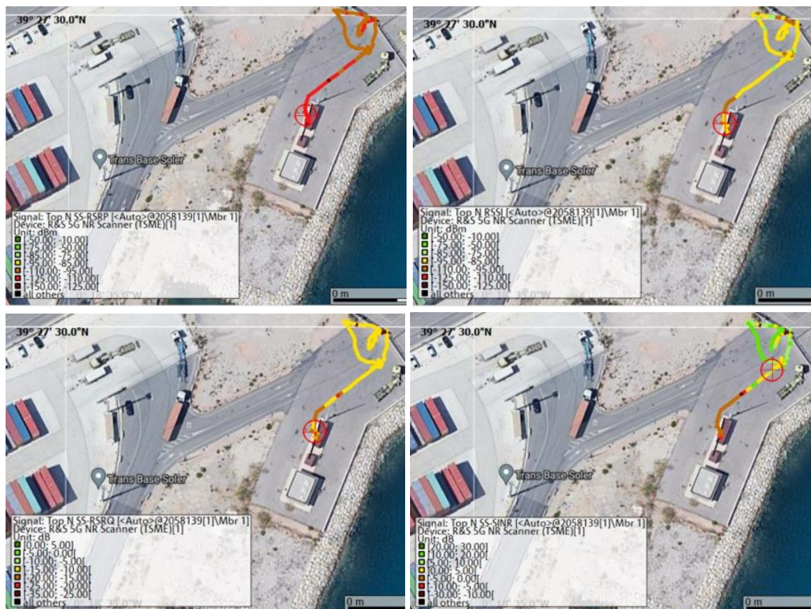
Figure 25 First drive test in the Valencia Port, results for RSRP (upper left), RSSI (upper right), RSRQ (lower left) and SINR (lower right)
