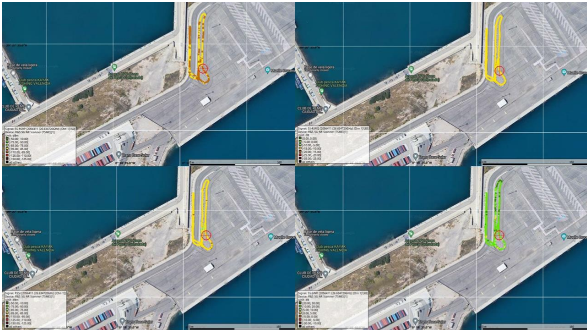
Figure 26 Second drive test in the Valencia Port, results for RSRP (upper left), RSSI (upper right), RSRQ (lower left) and SINR (lower right)
