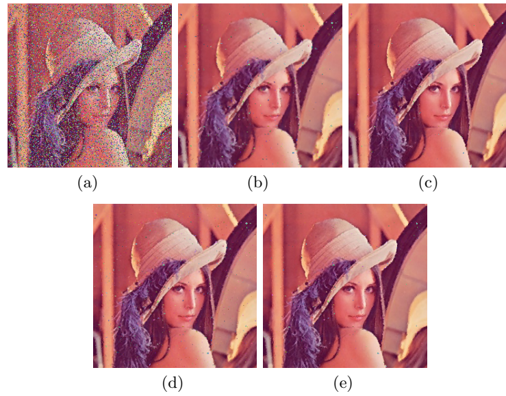
Fig. 9.6. Performance comparison: (a) Detail of Lenna image with 30% random-value impulsive noise, (b) VMF output, (c) FIVF output, (d) ASVMF output, (e) CFM' output.
