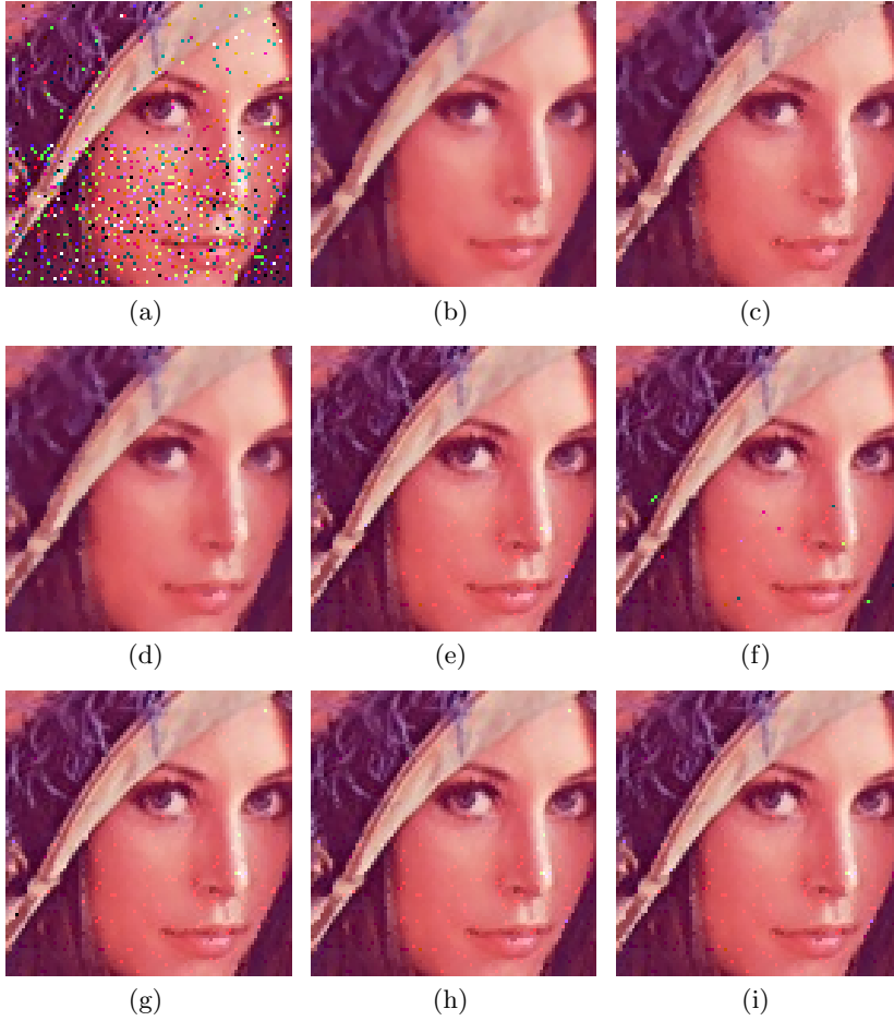
Fig. 8.2. Performance comparison: (a) Detail of Lenna image with 5% impulsive noise type I in the upper half and 25% impulsive noise type I in the lower half, (b) VMF output, (c) BVDF output, (d) DDF output, (e) FIVF output, (f) SAMF output, (g) SDF_{\sigma_F} output, (h) SDDF_{\sigma_F} output, (i) SDDF_{\sigma_F} output.
