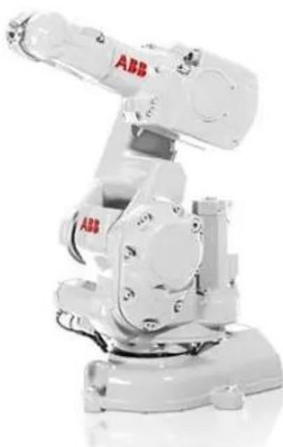
*Figura 33. Robot industrial ABB IRB 140*
