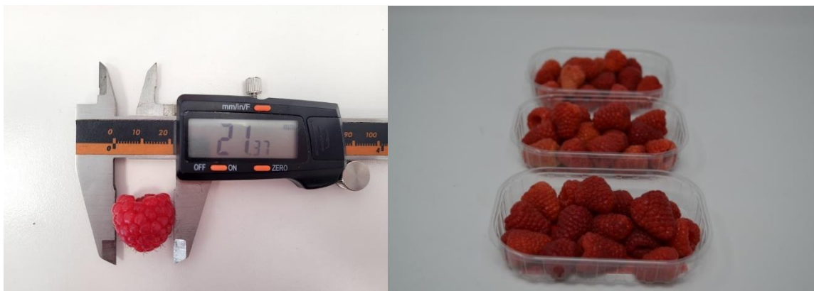
Figure 10 Materials used for harvest and fruit evaluation. Left: electronic digital caliper used for obtaining the measure of length and diameter of the berries; fruit from AMO-013 is shown on the picture. Right: Clamshells used for harvest. Picture shows first quality raspberries harvested from the selection AMO-022.
