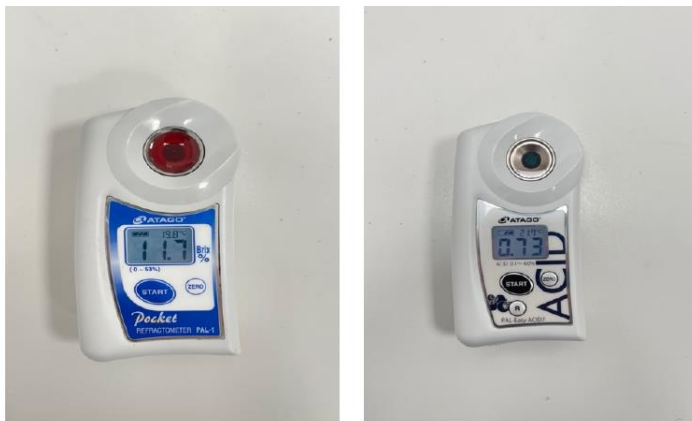
Figure 11 Instruments for solid soluble (on the left) and titratable acidity (on the right) determination.
