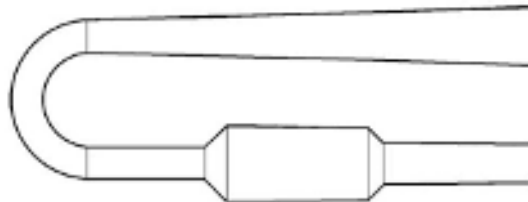
Figure 2.3: Pulsejet "U" Shape [5]
