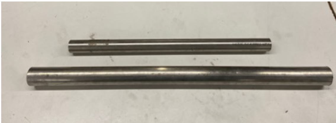
Figure 4.4: Intake and Exhaust ducts before being manipulated
