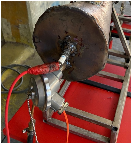
Figure 5.1: Thermocouple installed on the Pulsejet
