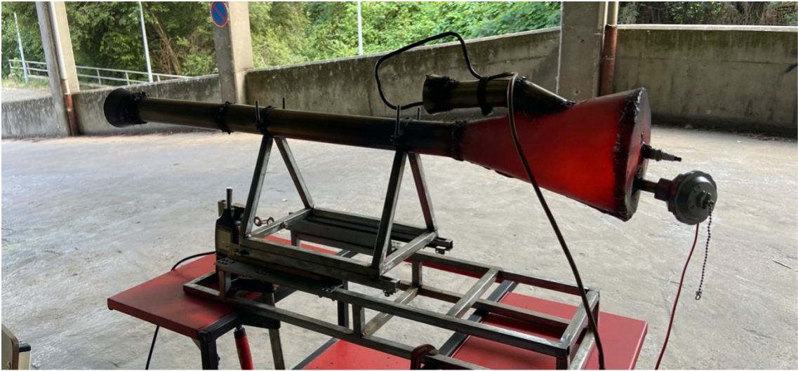
Figure 5.6: Combustion chamber heating
