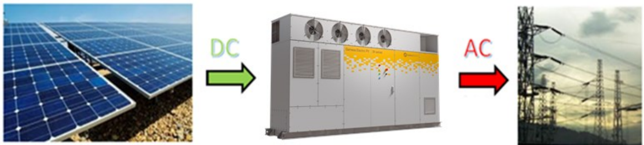
Fig 1. GamesaElectric PV 3X series inverter with connection to electrical grid
