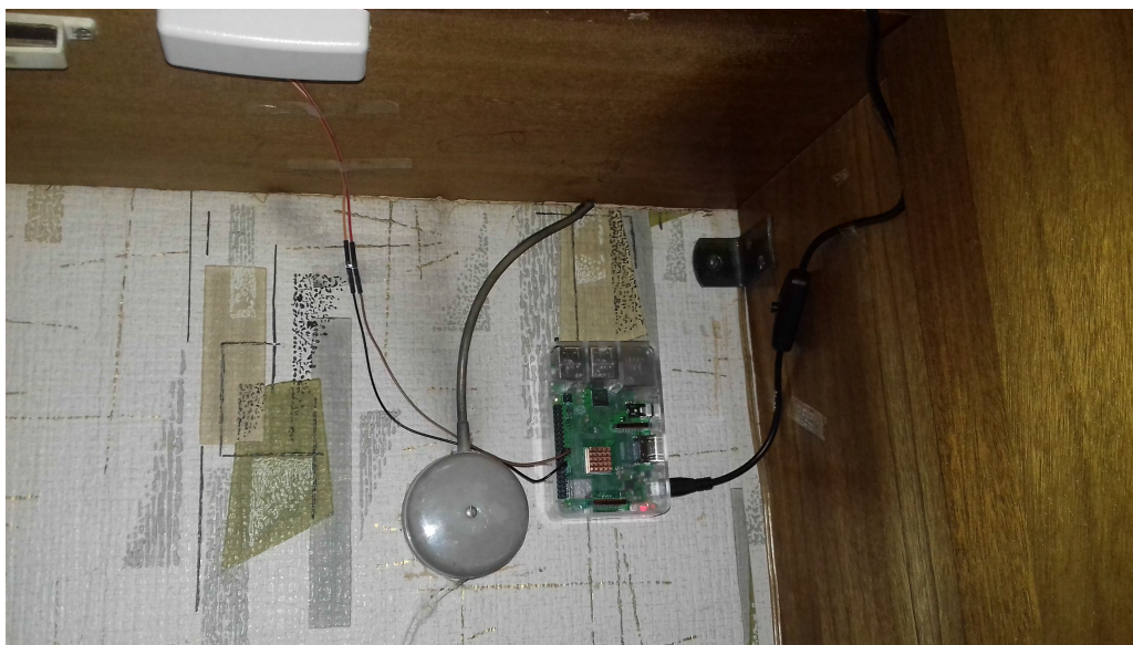
FIGURE 4. The Raspberry connected to the door sensor in the smart cupboard prototype.
