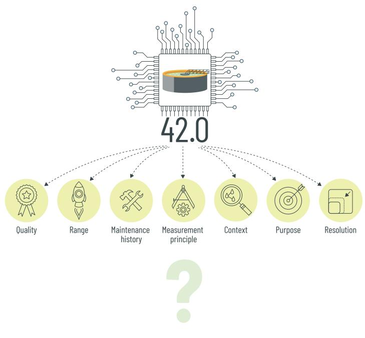
Figure 1. Can we interpret the provided measurement equal to 42.0? We need to know a lot more to evaluate the information contained in sensor signals. The kind of descriptive data we need for interpretation is known as "meta-data" and includes the purpose of measurement, the measurement principle, the temporal and measurement resolution, sensor maintenance history, indicators of signal quality, and the spatial and temporal context of the measurement.
