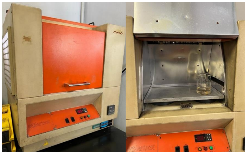
Figure 4. Solar box CO.FO.ME.GRA: and experimental procedure.
