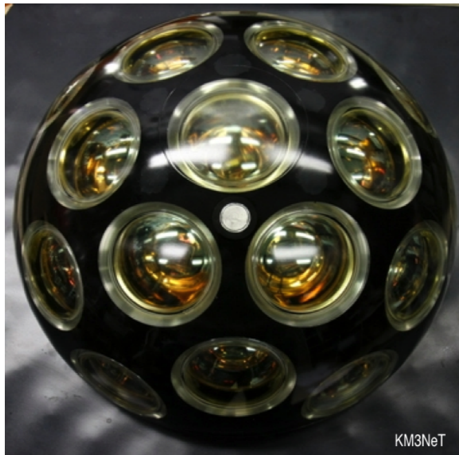
Figure 4.2.1: Photo of a a Digital Optical Module. Figure taken from [29].
