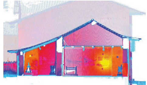
Fig. 7. Point-cloud image from the 3D database of Casa do Anhanguera in Brazil, highlighting the typical Portuguese colonial roof shape. The short digitization project involved local technicians and professionals to familiarize them with the technology and evaluate possible digital surveys on the most important vernacular buildings of the state of São Paulo (Image by the author).
