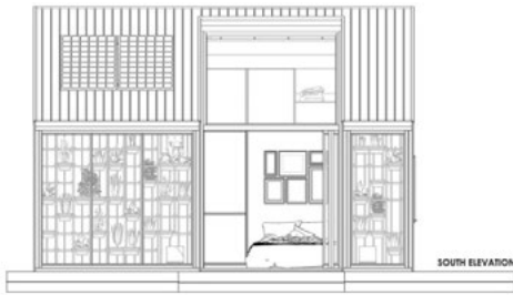
Fig. 3. The house south façade showing the integrated design of the hybrid Trombe wall and the green wall as passive systems.
