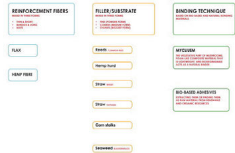
Fig. 4. The classification of the selected materials (natural fibres and fillers/substrates) and the targeted binding techniques.
