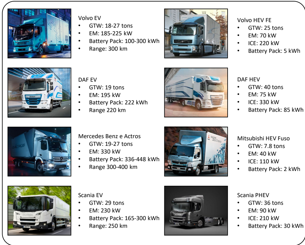
Figure 2-20. Examples of electrified HD trucks powertrain available in Europe.
