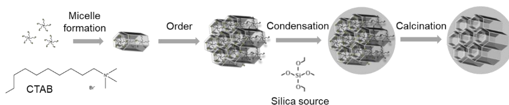
Figure 8 | Schematic representation of the synthesis of the mesoporous silica nanoparticles. First, a super-micellar template is formed in basic water solution. Next, the inorganic siliceous precursor tetraethylorthosilicate hydrolyses and condensates around the template. The final mesoporous inorganic MCM-41 scaffold, which presents cylindrical unidirectional empty channels arranged in a hexagonal distribution, is obtained by removing the surfactant template by calcination. CTAB: cetyl trimethyl ammonium bromide. Adapted from Hoffmann et al. Angew. Chem. Int. Ed. 2006, 45, 3216.
