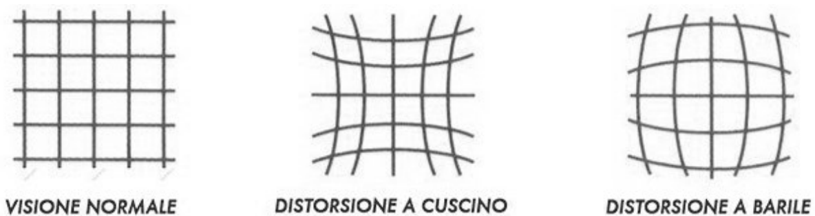
Fig. 51 - Diagrama de distorsiones. (Fuente: https://www.cinquephoto.com/wp-content/uploads/2013/02/Distorsioni-obiettivi.jpg ).
