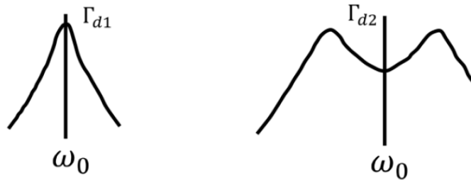
Figure 2.26: Group delay frequency response for one resonator (left), and for two coupled resonators (right).
