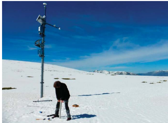
Figure 4. TNM and on-site manual sampling for the snow pole sampler.
