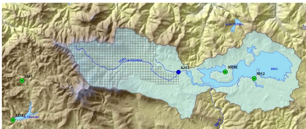
Fig. 4.6. ASTER hydrological model. Hajar river basin mesh (grey grid), Gauging Station (A203), rainfall stations (9008E, 9012) and temperature stations (2225, 2232)
