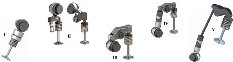
Figure 2.13: Typical valvetrain configuration for light-duty application. Source: [53].
