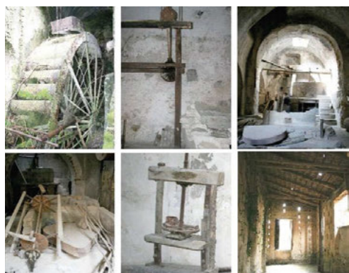
Fig. 4. Amalfi, Valley of Mills. Processing machinery and rooms of the Di Pino paper mill (iron wheel; fuso , pila , tino , torchio or strettoja , and spanditoio ).
