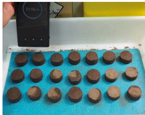
Fig. 2. Sample of the capillary water absorption test (Source: Medina Lorente, 2020).
