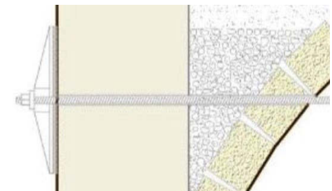
Fig. 22. Steel tie-rod in a barrel vault (Source: Caleca, 2018)
