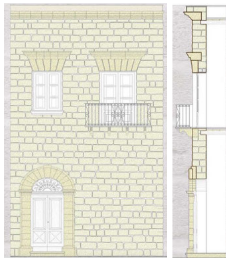
Fig. 9. Masonry wall with arch systems (Source: Caleca, 2018)
