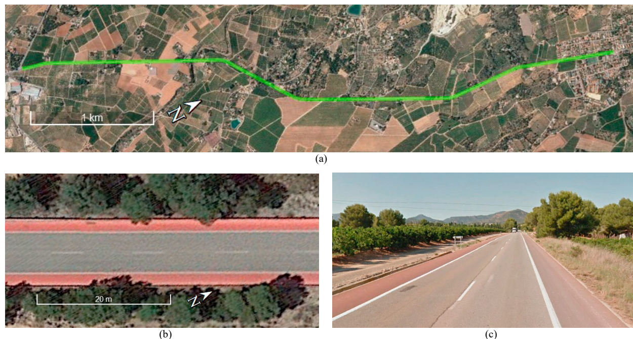
Fig. 2 - Road segment and cross-section characteristics: (a) road segment in CV-310 analyzed; (b) aerial view of a section of the rural road; (c): driver's view along a straight road section.
