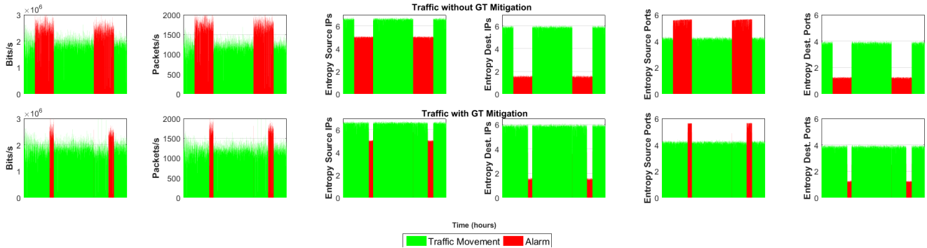
Figure 17: Hexa-dimensional IP flow view of the analyzed SDN, with two DDoS attacks based on 15 hosts, before and afterwards the procedures of detection and mitigation utilizing CNN and GT.
