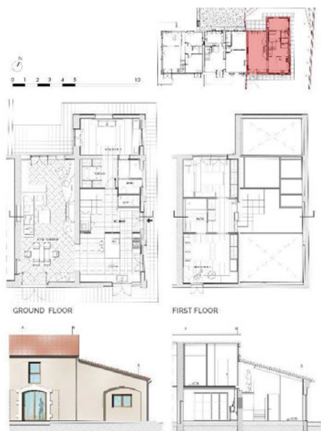
Fig. 4. The Unit 3 project: ground floor, first floor, main façade, longitudinal section. On the left side of the building: the barn. On the right, the peasant house. (Source: Li Puma, 2021)
