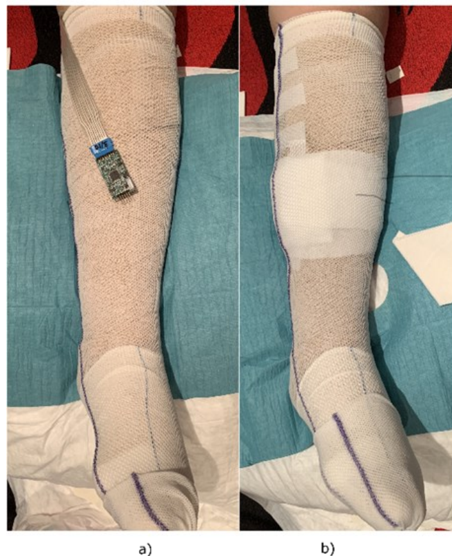
Figure 19. Placement of the system in the wound dressing. (a) Sensors applied under a finished bandage; (b) protection of the data acquisition system to avoid damaging the device and the patient during their activity.
