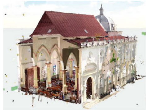
Fig. 4. Three-dimensional model by laser scanning. (Source: elaboration by Gómez Mejía, 2020).
