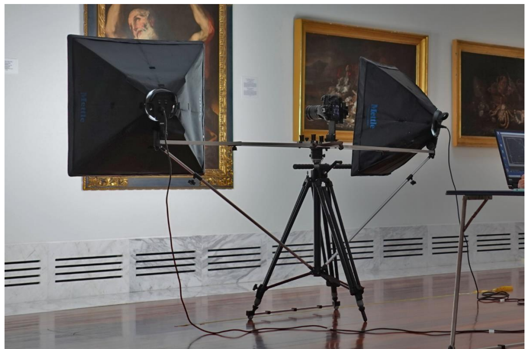
Figure 10. Lighting mount to attach the lighting system to the tripod.
