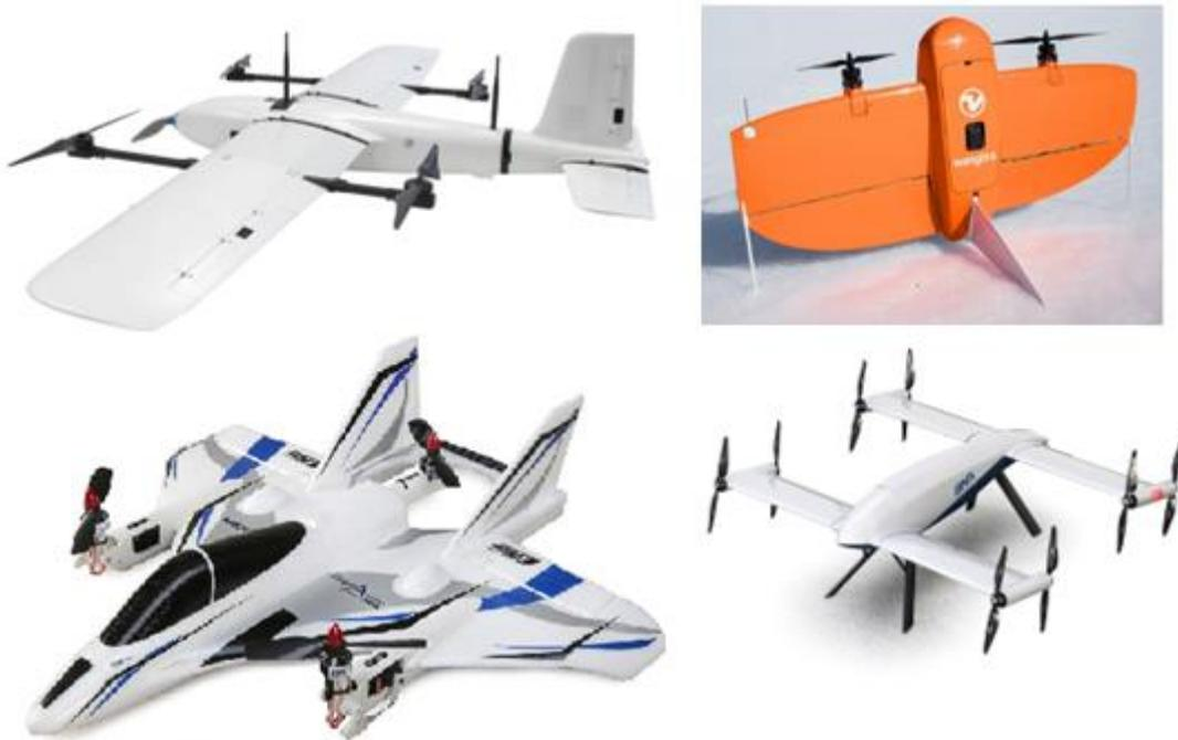
Figura 2.3. Quad plane, tail sitter, tiltrotor y tilt wing, respectivamente. [16,13,14,15]
