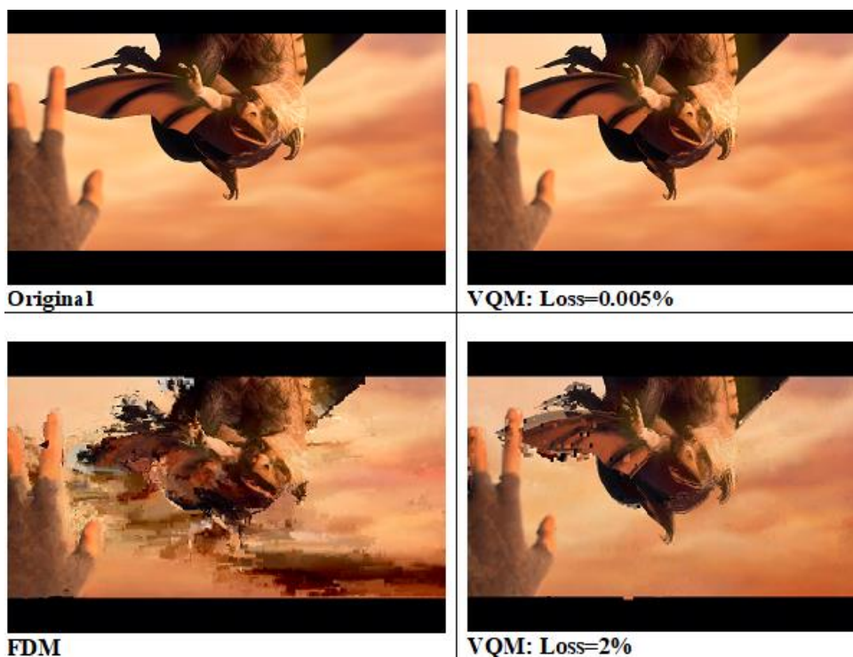
Fig. 11. Impact of setting the TwoLLWPs by packet loss rates (0.005% or 2%) against FDM.
