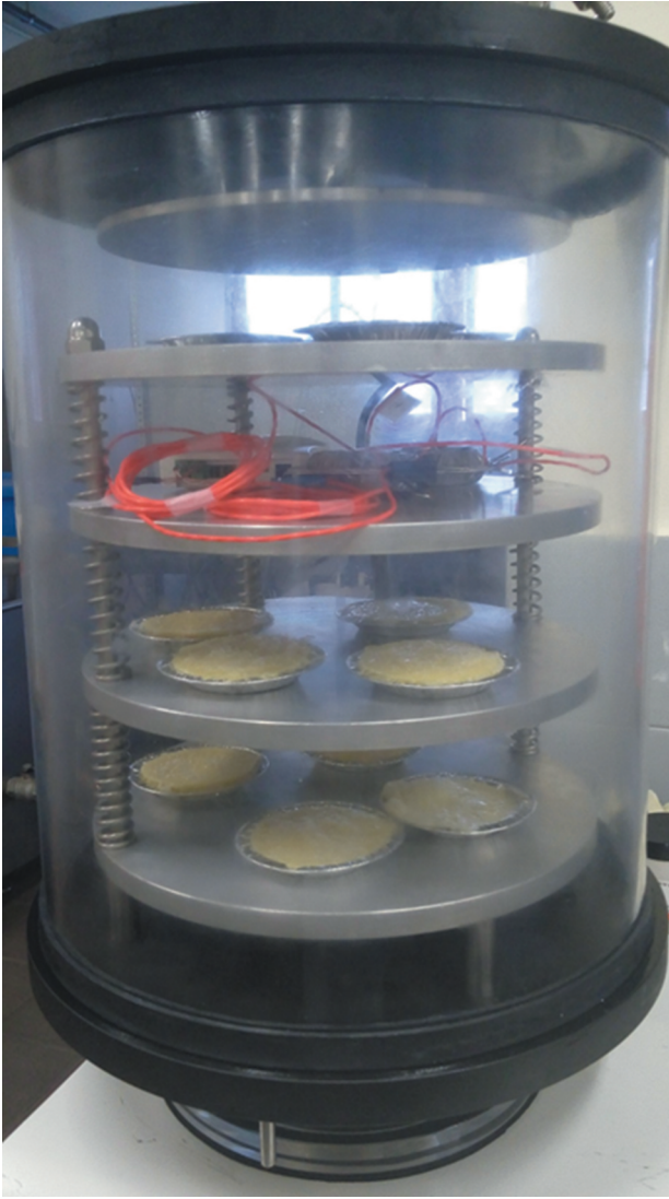
Figure 1. Freeze drying chamber for orange juice based cake experimental dynamics.
