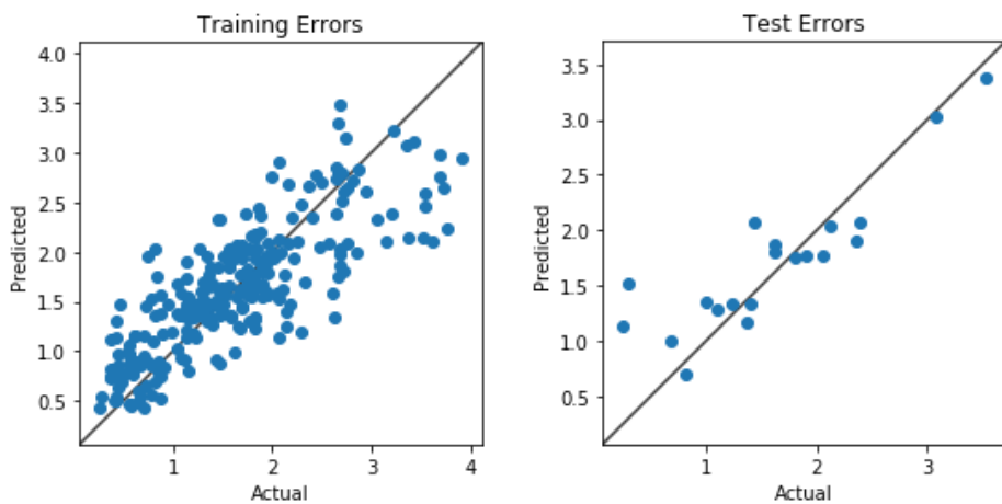
Figure 9. Polymeric pigments (AU) regression plots, calibration model (left) and validation set (right).
