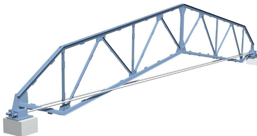
Figure 2. A new type of prestressed arched truss with a tie member offered by the authors.
