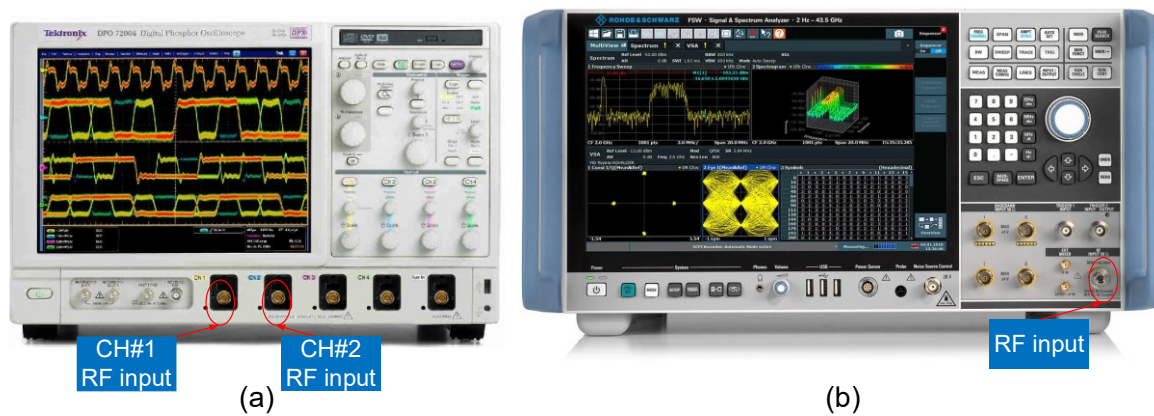
Figure A.7. Signal analyzers employed in this Thesis: (a) Tektronix DPO72004CC and (b) Rohde & Schwarz FSW43.
