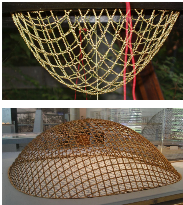
Figure 25. Hanging chain net with close flat boundary, and inverted funicular model of Frei Otto's Deutsche Bauausstellung gridshell. Essen, 1962. ©Author's photographs
