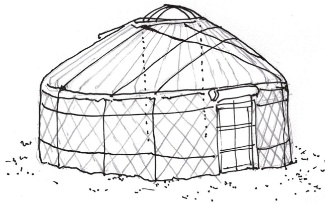
Figure 9. Yurt. Inner frame and outer felt covering tightened with ropes. ©Author's drawing
