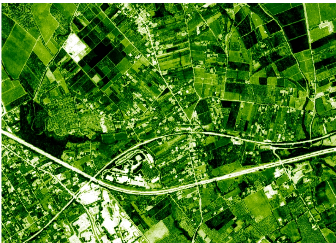
Image 12: NDVI zone obtained with Band Math, and applying the Green/White linear colour scheme
