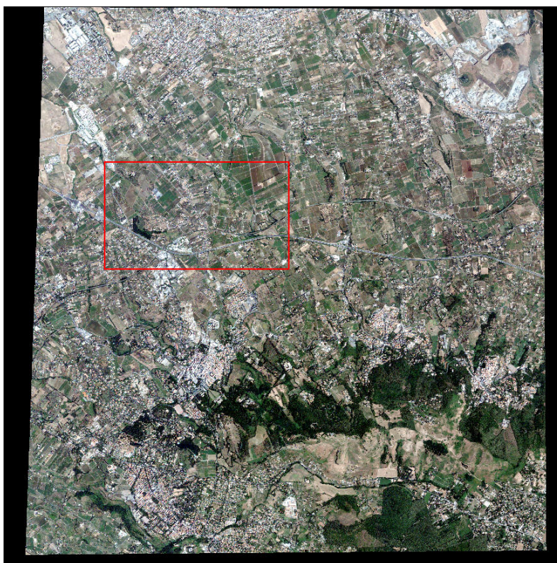
Image 3: Example of multispectral QuickBird image used, in true colour composition (R,G,B)=(Band3,Band2,Band1)
