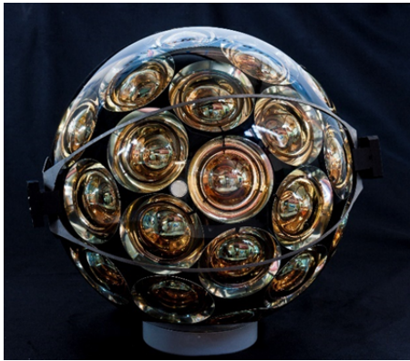
Figure 3. Bottom view of an optical module, illustrating its large effective and segmented photon detection area. On the left of the middle PMT, the acoustic piezo sensor used for positioning measurements (see section 3.2) is visible. The titanium collar required for mounting in a detection unit is also visible.
