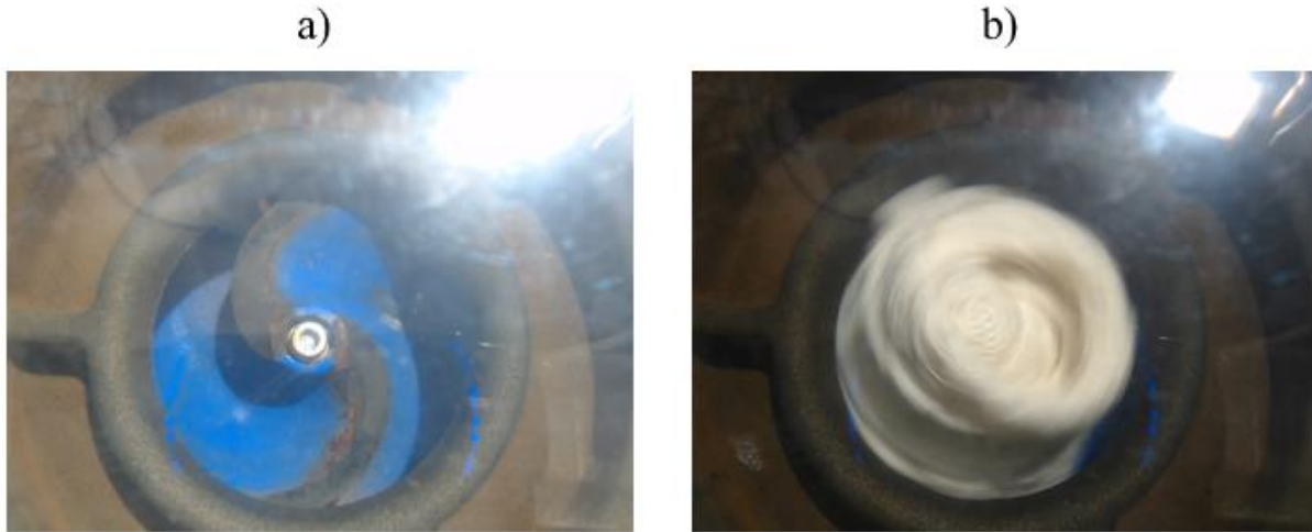
Figure 4.5: Standstill ESP impeller in healthy condition (a) and running with clogging (b)
