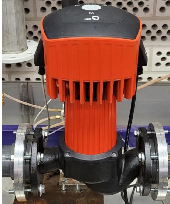
Figure 4.1: Picture of the measured wet-rotor pump with 800 W
