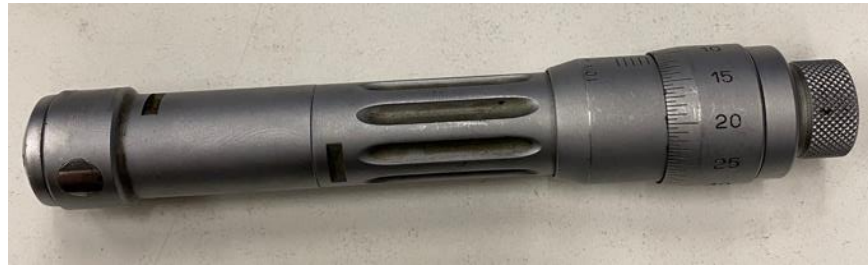
Figure 4.8: Measurement device for measuring the bushing diameter
