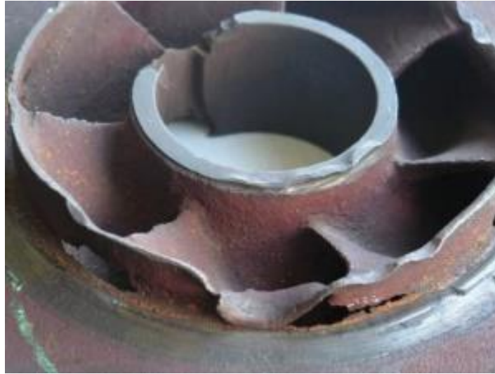
Figure 2.9: Damage to an impeller due to cavitation (Milan, 2004)
