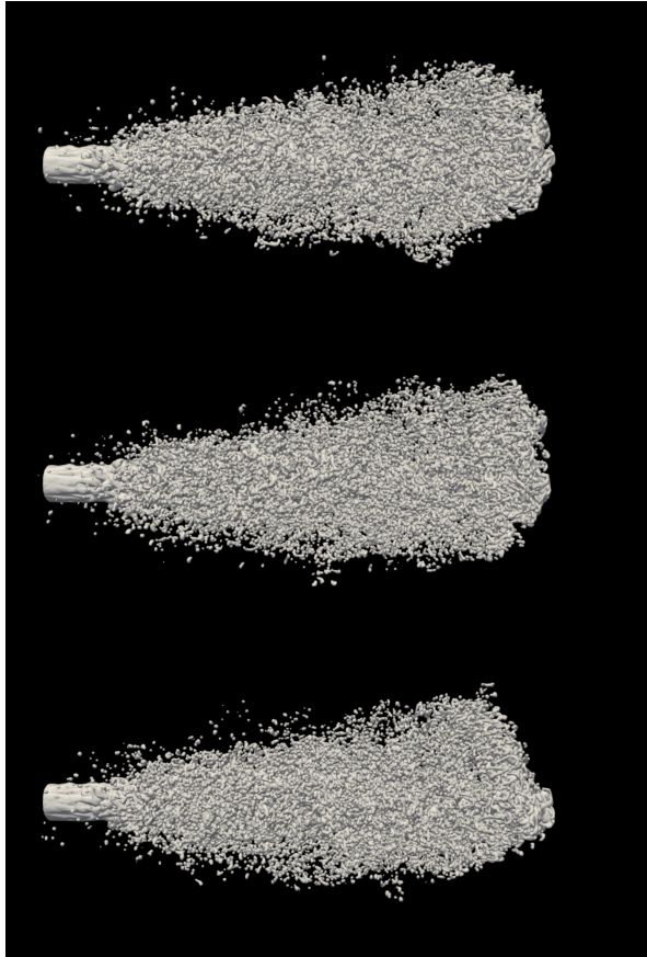
Figure 6.1: Spray morphology during the transient state at T = 12.5 \mu\text{s} . Increasing Weber number from top to bottom.
