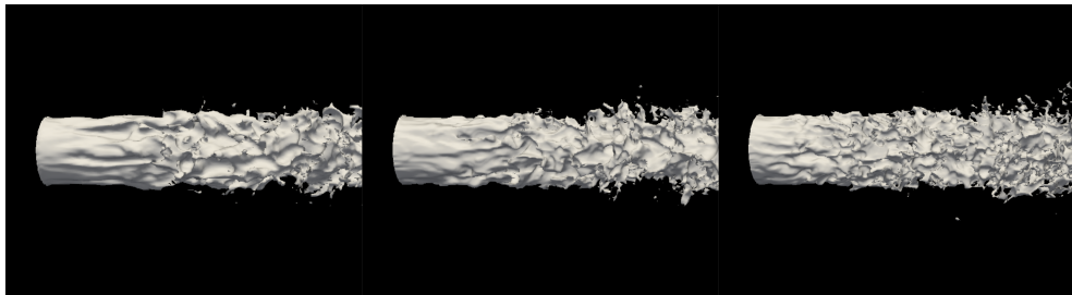
Figure 5.3: Spray core extracted from the full spray at T = 150 \mu\text{s} . Increasing Reynolds number from left to right.
