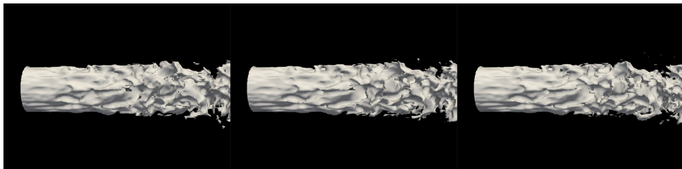
Figure 6.3: Spray core extracted from the full spray at T = 150 \mu\text{s} . Increasing Weber number from left to right.
