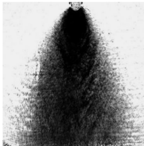
Figure 1.14: Result of an effervescent spray from Linne et al. [68].
