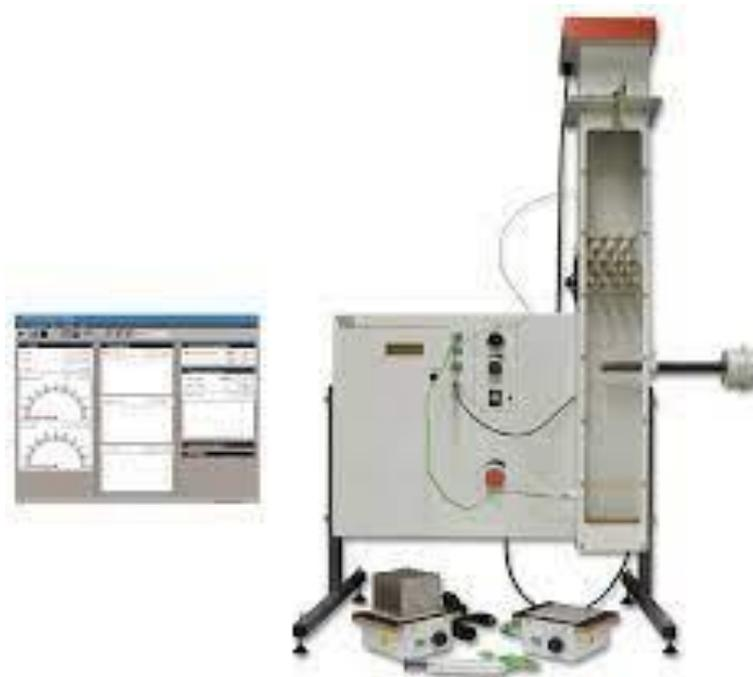
Figura 9. Equipo TD-1005 “Free and Forced Convection”
