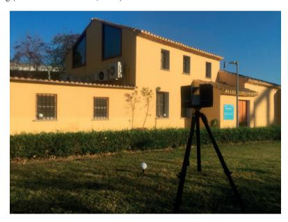
Figure 1. 3D laser scanner and placement of spheres in the farmhouse.
