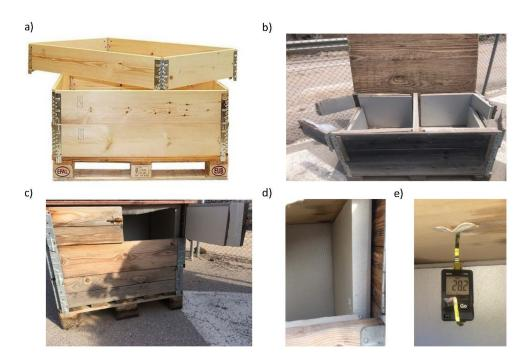
**Figure 1.** Euro-pallet support. (**a**) three wooden rectangular articulated bodies (image courtesy of www.rotomshop.es accessed on 4 January 2020); (**b**) interior space divided into two compartments; (**c**) access door; (**d**) expanded polystyrene insulation; (**e**) thermo-hygrometric TESTO 174H sensors/data-loggers hanging on the wood ceiling.
