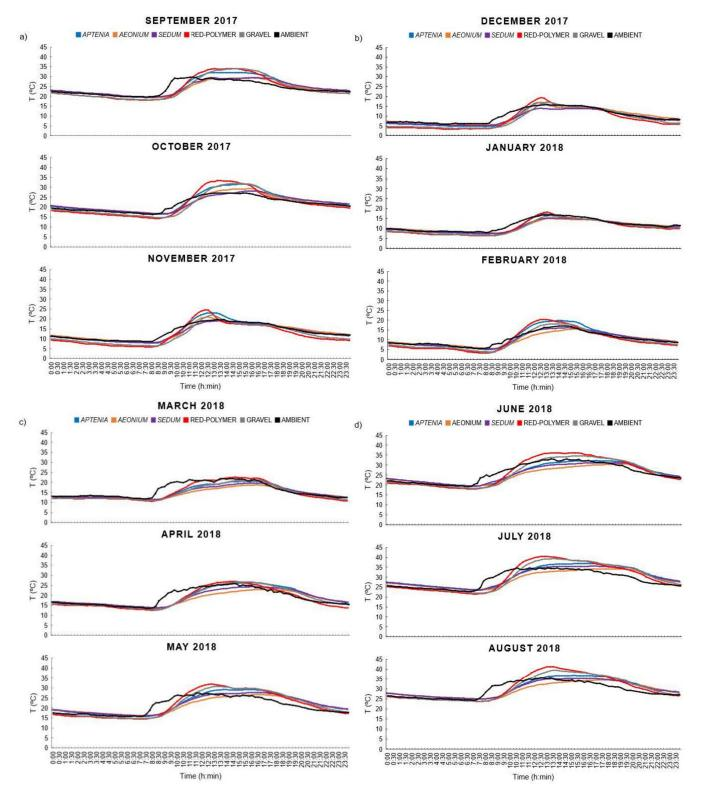
**Figure 4.** Average temperatures registered every 15 min during the day in the ambient, and under different covers: conventional (red-polymer, gravel) and green (*Aptenia, Aeonium* and *Sedum*) in (**a**) autumn 2017, (**b**) winter 2017–18, (**c**) spring 2018, and (**d**) summer 2018.
