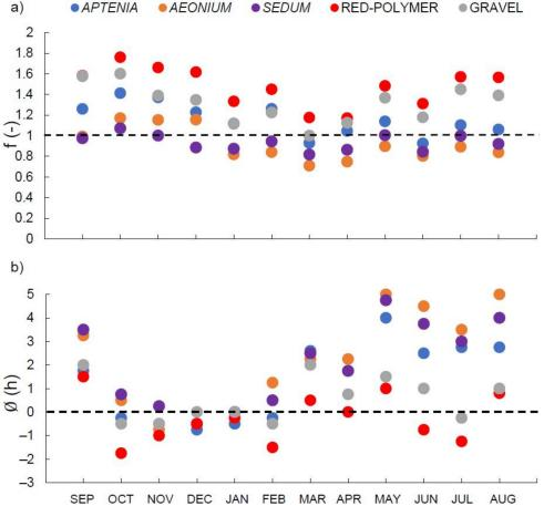
**Figure 5. a)** Decrement factor and **b)** time lag for conventional (red-polymer and gravel) and green covers (*Aptenia, Aeonium,* and *Sedum*). Dashed lines are plot as a reference with respect to ambient ( $f = 1, \emptyset = 0$ ).
