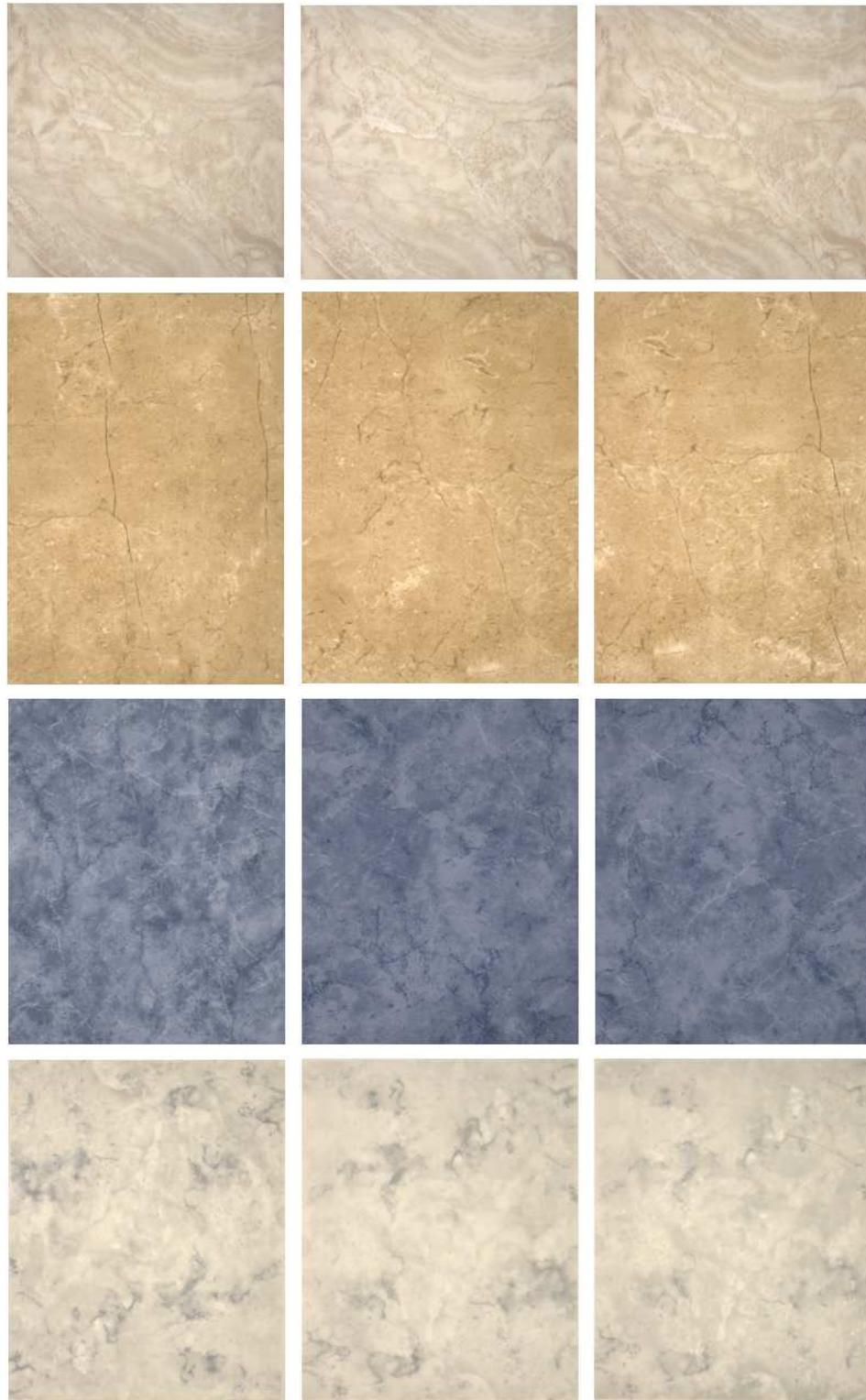
Figure 3.6: VxC TSG granite samples. From up to down; three samples of berlin, oslo and lima models, each one corresponding to a different surface grade.
