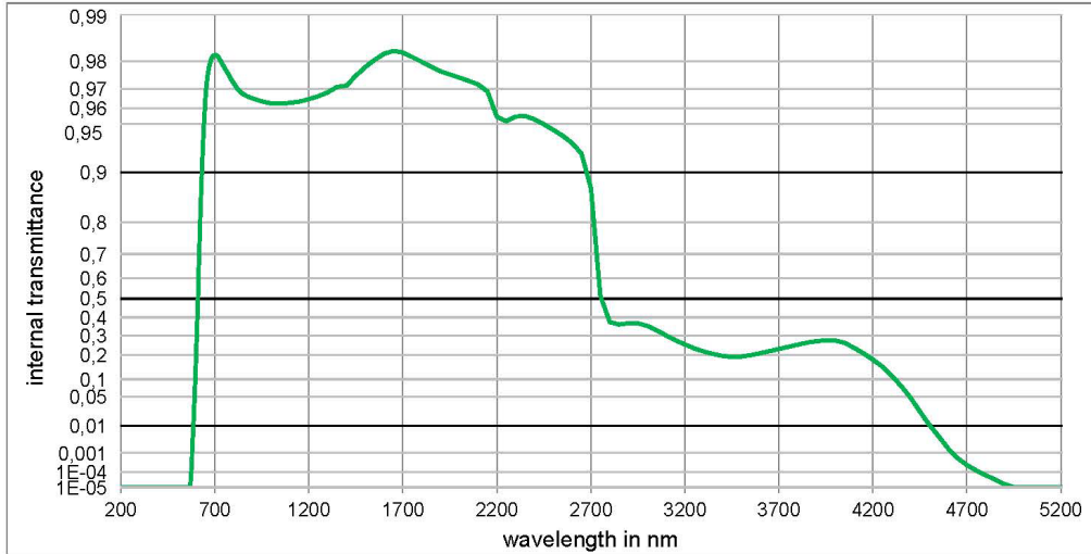
Internal transmittance \tau_i at reference thickness The internal transmittance values, tabulated and graphically represented, are reference values only
