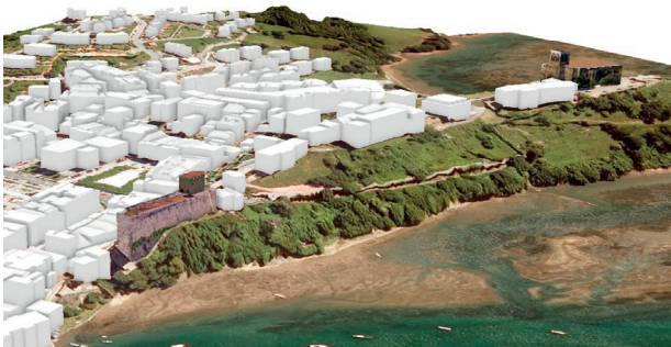
(c) San Vicente de la Barquera in LoD2 and LoD3 (castle and church).
