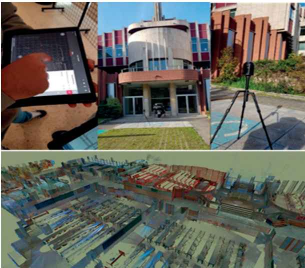
Figure 10 | 3D laser scanning process and Point cloud obtained (visualized in Revizto software).
